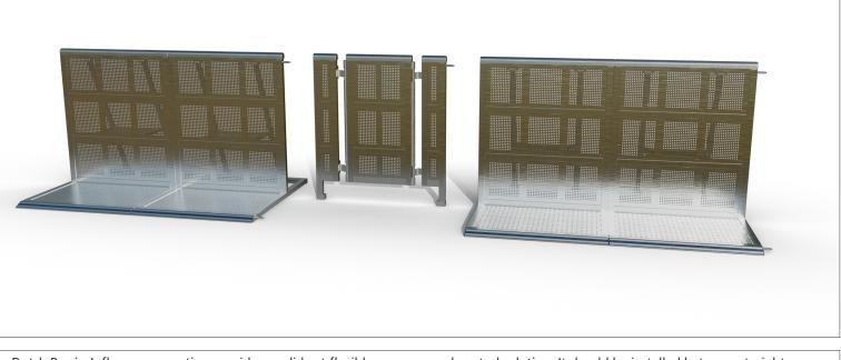
Dutch Barrier's flex corner section provides a solid yet flexible corner crowd control solution. It should be installed between straight sections only. Although it withstood the same 5kN/m test condition, we recommend only using it in reduced maximum crowd pressure areas due to the lack of braces and treadplate a.o. They are stored and travel per 15 in an all-new handling-friendly dolly system.
