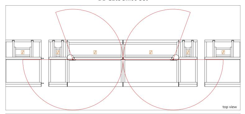
Among the most intricate of gates, the Dutch Barrier's 3m00 gate set consists of two doors and two customized half-straight sections, opening from the centre towards both left and right sides. With both doors swinging inward and outward, they can function as utility gates or blow-out gates, ensuring high-volume egress following a show or event.
