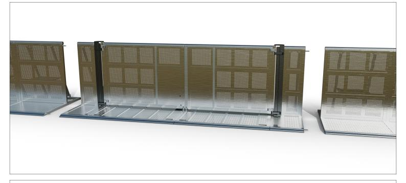
The Dutch Barrier's 3m00 gate set is the most intricate of gates. It opens from the centre. Its locking system, integrated with ball bearings in the treadplates, ensures staff can unlock it even under pressure. Once set up, staff may remove the treadplates to allow vehicle passage. It's a multi-purpose utility gate which can double as an emergency exit at a suitable location.
