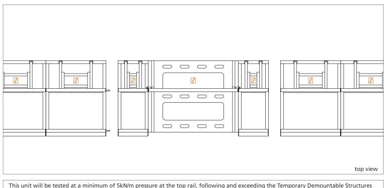
This unit will be tested at a minimum of 5kN/m pressure at the top rail, following and exceeding the Temporary Demountable Structures Edition 4 guidelines by the Institution of Structural Engineers (ISE). TUV reports for each test will be available at Dutch Barrier & Dutch Barrier Services upon request.
