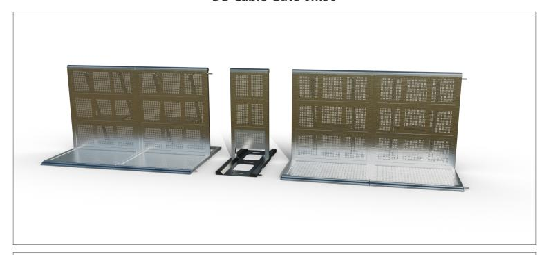
Dutch Barrier's cable gate 0m50 consists of a treadplate and a removable upright. It does not require half-straight sections on either side. It provides a rock-solid crowd control solution in need of a small cable run. When running cables or smaller cable ramps, simply take out the upright by removing the two top bolts.
