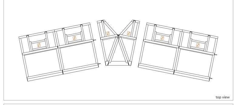
An infill secures a vario corner at a specific angle, providing continuity to the treadplate, reducing the risk of tripping and minimizing the chance of the barrier overturning with more people standing on the treadplate. TUV has determined that the least robust configuration, a vario corner section without an infill, meets the 5kN/m ISE requirement. Therefore, it will be even stronger combined with infills.
