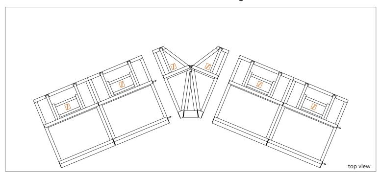
An infill secures a vario corner at a specific angle, providing continuity to the treadplate, reducing the risk of tripping and minimizing the chance of the barrier overturning with more people standing on the treadplate. TUV has determined that the least robust configuration, a vario corner section without an infill, meets the 5kN/m ISE requirement. Therefore, it will be even stronger combined with infills.
