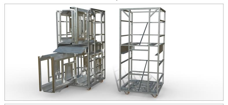
Dutch Barrier's Dolly LUG is designed for efficient storage and transport of LUG sections, with four internal passages for secure positioning. Each set can hold either three full and two half sections, or four full sections. Its angled upper compartment ensures parts roll smoothly into place without falling out, while the removable access gate allows quick loading and unloading for fast, organised handling on site.
