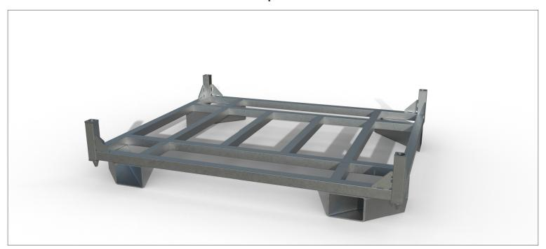
Dutch Barrier's Transport Pallet is designed for safely stacking and securing two Dutch Barrier dollies on a curtain sided trailer. By lifting the wheels clear off the trailer floor, unwanted movement during transport is minimized, ensuring a stable and secure load. Its robust frame prevents sliding and provides a safe, efficient solution for road transport of barrier systems.
