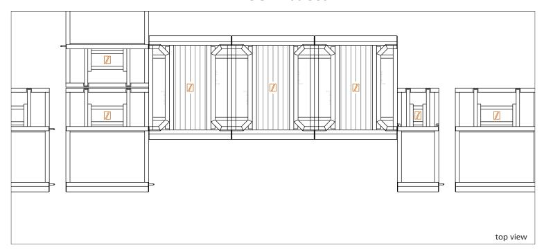
Once assembled, line-up gates create 0m50 wide walkways, separated by bumper units. A standard set comprises three bumpers, two half bumpers to serve as end caps and four treadplates, forming four consecutive walkways. Inside the bumpers, staff can for eample safely perform tasks like ticket-checking. An extension set of four bumpers and treadplates is also available.
