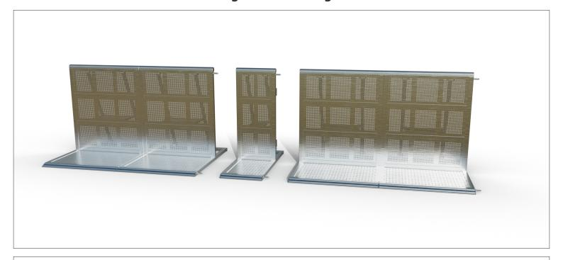
Dutch Barrier's Straight 0m50 - Hinge Blocks also doubles as a gatepost for several cablegate and gate options when hinges are in use. Therefore, it only has a threadplate pin and requires a mandatory top bolt instead. If required, the Straight 0m50 is available with a top pin and without hinges. They are stored and travel per 14 units in an all-new handling-friendly dolly system.
