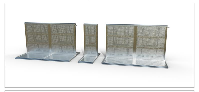
Dutch Barrier's Straight 0m50 – Breaker is designed for quick and flexible setup changes at multi-day events, where barrier lines may need to be adapted overnight. Because it has no pin, this 0m50 section can be slid in and out of the barrier line once unbolted, allowing easy layout changes without compromising strength or alignment. Its orange step provides clear visual recognition for crew during operation.
