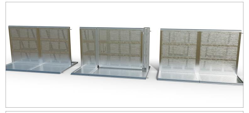
Dutch Barrier's Gate 1m50 – Right (set) is the right-opening version of the 1m50 Gate and can be configured for two setups. In the front-of-stage setup, the gate only opens towards the audience, making it suitable for high crowd pressure areas. In the low-pressure setup, it opens in both directions and can function as an efficient blow-out gate.
