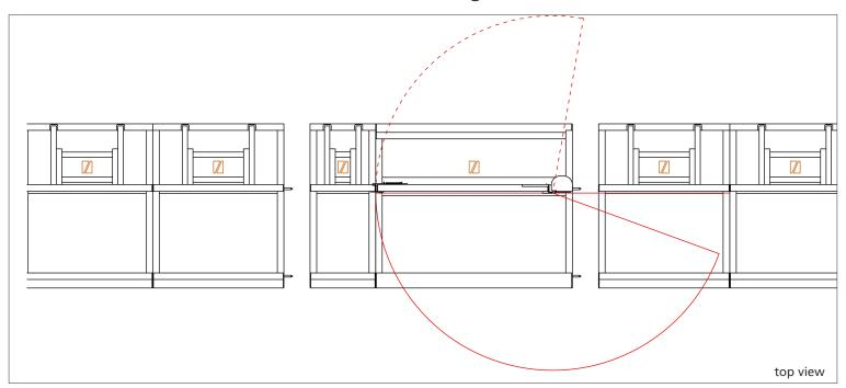
Testing was done at a minimum of 5kN/m pressure at the top rail, in high pressure setup, following and exceeding the Temporary Demountable Structures Edition 4 guidelines by the Institution of Structural Engineers (ISE). TUV reports for each test are available at Dutch Barrier & Dutch Barrier Services upon request.
