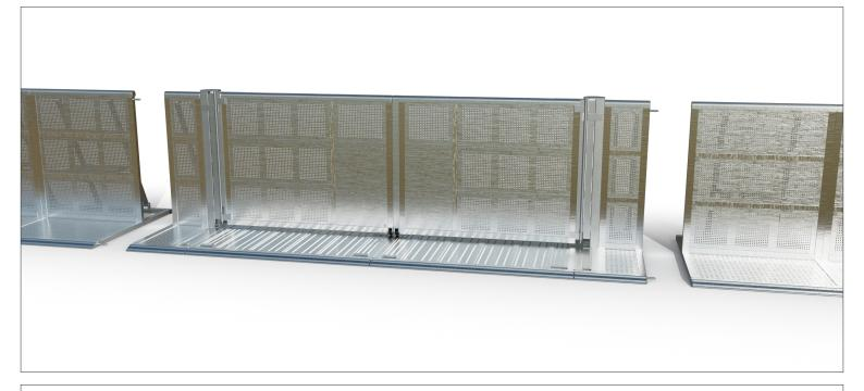
Dutch Barrier's Gate 3m00 (set) is the most intricate of gates. It opens from the centre. Its locking system, integrated with ball bearings in the treadplates, ensures staff can unlock it even under pressure. Once set up, staff may remove the treadplates to allow vehicle passage. It's a multi-purpose utility gate which can double as an emergency exit at a suitable location.
