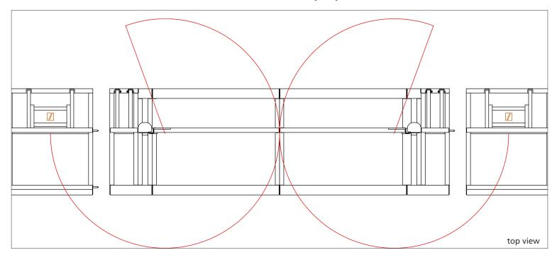
Among the most intricate of gates, the Dutch Barrier's 3m00 gate set consists of two doors and two customized half-straight sections, opening from the centre towards both left and right sides. With both doors swinging inward and outward, they can function as utility gates or blow-out gates, ensuring high-volume egress following a show or event.
