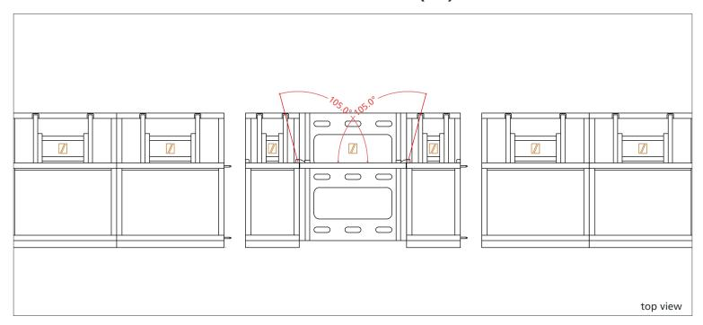
Testing was done at a minimum of 5kN/m pressure at the top rail, following and exceeding the Temporary Demountable Structures Edition 4 guidelines by the Institution of Structural Engineers (ISE). TUV reports for each test are available at Dutch Barrier & Dutch Barrier Services upon request.
